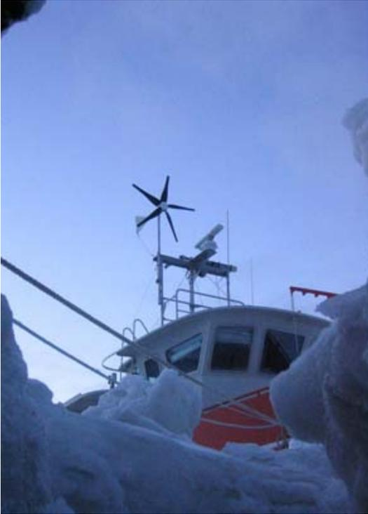
Launched in October 2004, the 18.50-metre long Aurora Magnetica is the first of a new generation of small aluminium hulled research ships purpose-designed for the exploration of the Arctic's remotest regions, where its low 1.40-metre draft and ability to manoeuvre in shallow waters opens up routes currently closed to conventional ice-strength vessels.
