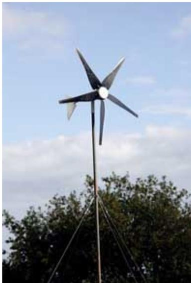
system is designed to generate real electricity from a light breeze onwards – and over 1KW in a stiff breeze (at wind speeds of 8.5 – 12 metres/sec) - and with a cost of just £695 for the basic turbine provides an average payback period of around five-years.
