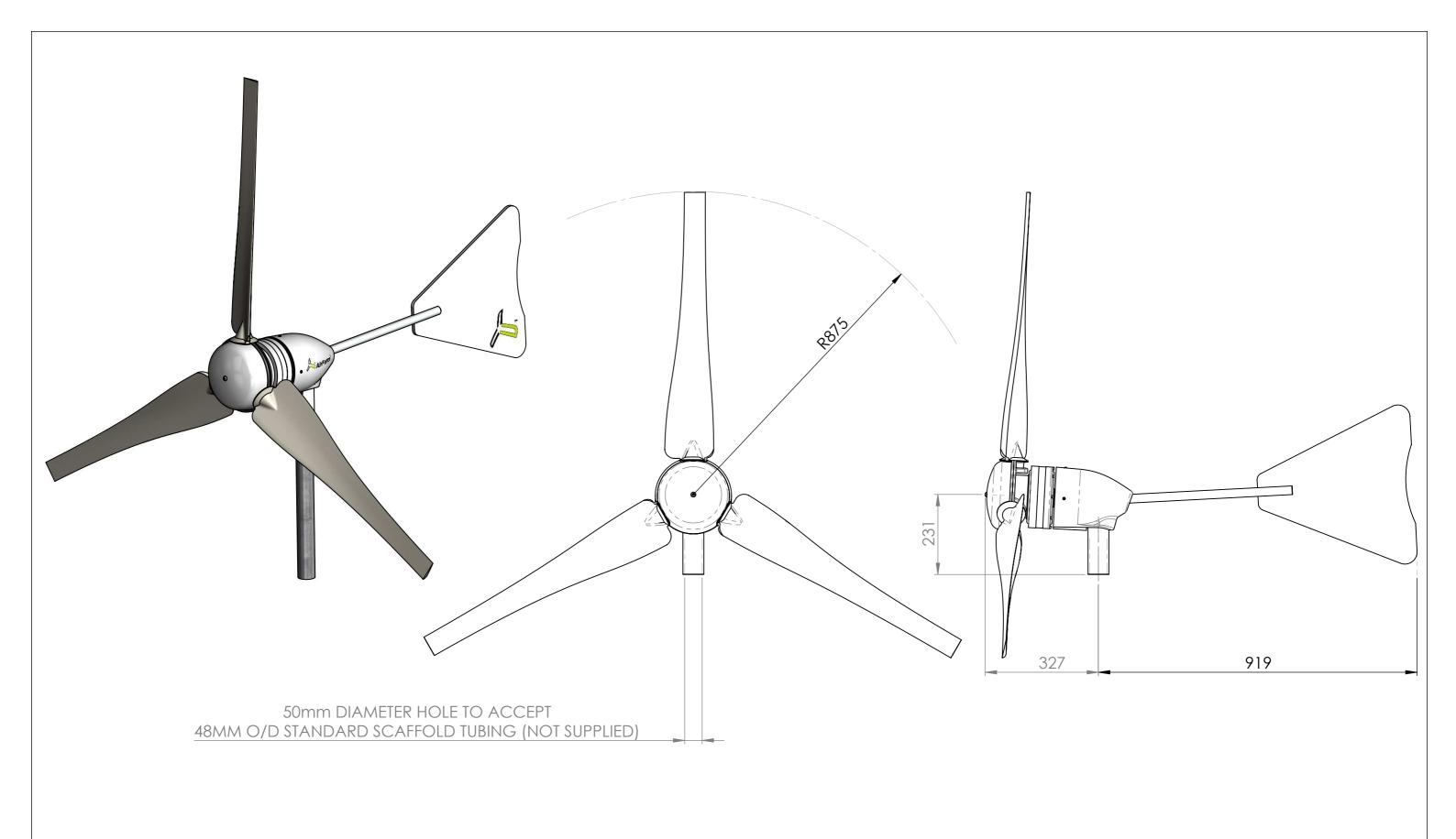
SWEPT AREA - 2.4m2 NORMAL OPERATION SHAFT LOAD - 274 N HIGH WIND LOADING (52.5m/s) - 610 N
